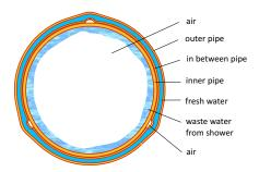
As a result of the high velocity of the waste water streaming along the inside of the inner pipe no fouling occurs. This means that normally no cleaning is necessary. However, greasy water and shaving gel can foul the inner tube. Avoid causing this. Flush now and then with water and soap.
